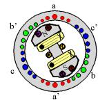
The ratio of phasor (vector) sum of induced emfs per coil to the arithmetic sum of induced emfs per coil is known as *pitch factor (Kp)* or *coil span factor (Kc)* which is always less than unity.
