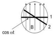
$$E (t) = N \frac{d\Phi(t)}{dt} = N B D L \frac{d \left[\cos(\omega t)\right]}{dt} = N B D L \omega \sin(\omega t)$$
